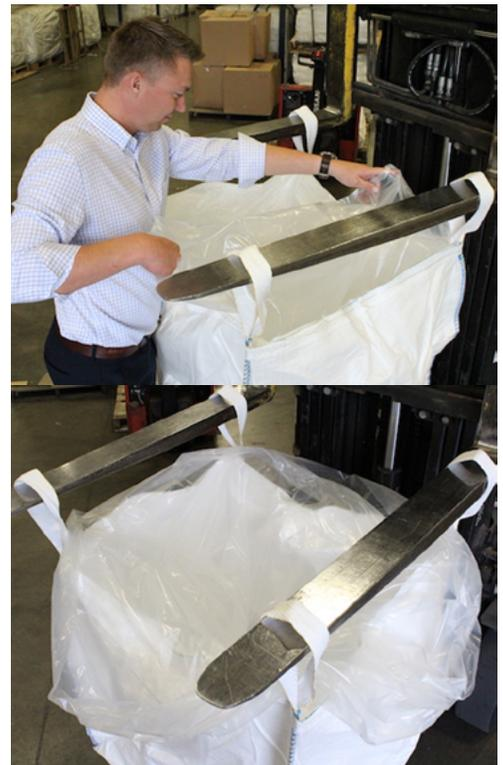
*Shown above are 2 pictures of liners inserted into bulk bags*
